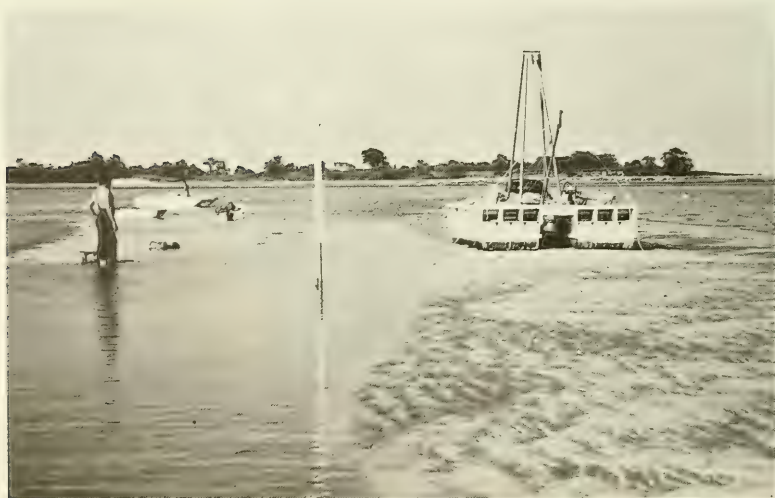
Figure 7. Barge on the Crest of a Sand Wave. Long staff in center is a tide gauge. The pipe to the right of the gauge is part of the diver support system.
